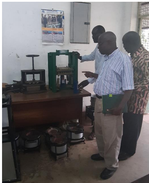
The OWC Liason Officer to NARO, Major Peter Murara Rwego admiring briquetting machine developed by NARO. The machine can make 49 bricks per minute from saw dust.
